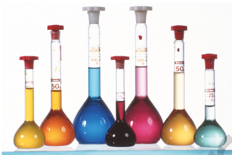
FIGURE 7.3.3 Volumetric flasks of various sizes are used to prepare standard solutions.
