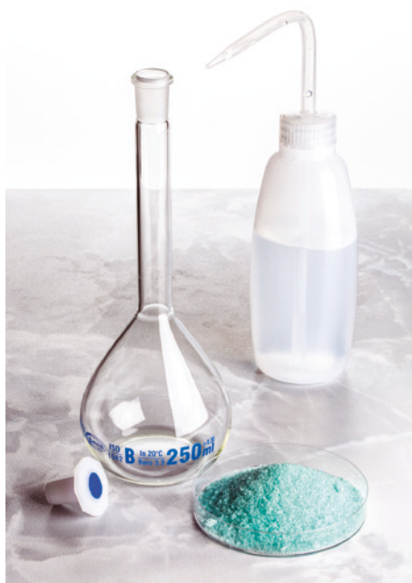
FIGURE 7.3.1 Apparatus and materials needed to prepare a standard solution. The measured mass of solid will be dissolved in water in a volumetric flask to make an accurate volume of solution.
